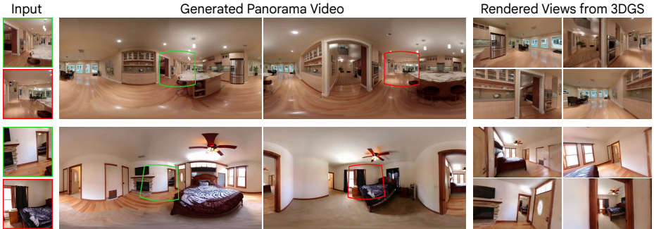
Fig. 10: Qualitative results of 3D scene reconstruction. Given an input monocular video (left), 360Anything outpaints the whole 360° viewpoint (middle), from which we can optimize a 3DGS (right). This allows fly-through exploration of the entire 3D scene.
